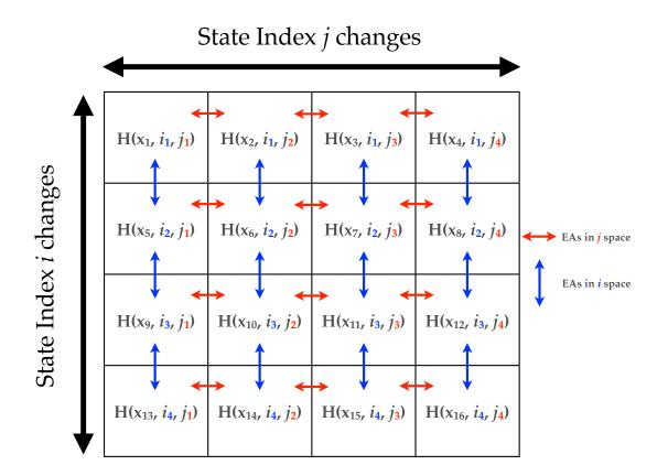
Figure 21.2.: Schematic showing exchange attempts (EAs) in multi-dimensional REMD simulations. Exchange attempts are indicated by the colored arrows, where red arrows indicate exchange attempts between replicas in a group of the dimension defined by the j state parameters. Blue arrows indicate exchange attempts between replicas in the dimension defined by the state parameter i. Figure taken from ref. 474.
