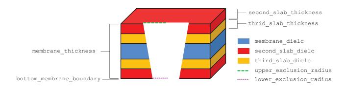
Figure 34.5.: Parameters for definition of implicit membrane in MM-PBSA calculations.
