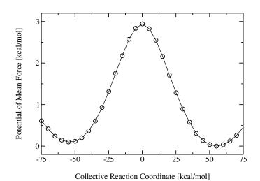
Figure 8.3.: Potential of mean force for the intramolecular proton transfer in malonaldehyde as obtained from a series of umbrella sampling simulations along an energy gap RC. The distributions of the RC from all the windows are combined using the WHAM procedure.
