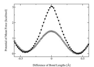
Figure 8.4.: PMFs as a function of the difference of bond lengths involving the proton with the donor and acceptor oxygens in malonaldehyde. The ▼curve is from classical EVB, while the ⊙ curve is from EVB/PIMD.
