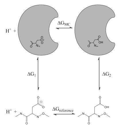
Figure 22.1.: Thermodynamic cycle used in CpHMD simulations. The energy difference between the two protonation states computed by sander is equal to the difference  $\Delta G_1 - \Delta G_2$  and  $\Delta G_{MC} = \Delta G_2 - \Delta G_1 - \Delta G_{reference}$  is used to evaluate the Metropolis Monte Carlo criteria for the proposed change in protonation state(s).
