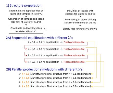
Figure 34.8.: Internal TI workflow of FEW consisting of structure preparation, equilibration simulations, and production simulations.
