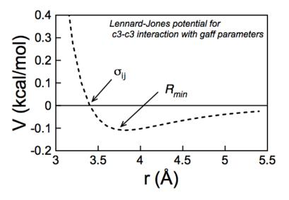
Figure 14.2.: Example of Lennard-Jones potential: the used data are those for the c3 atom type in the gaff force field (vdW radius  $R_{min}$ = 1.908 Å,  $\varepsilon$  = 0.1094 kcal/mol)
