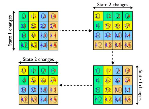
Figure 21.3.: Replica arrangement in multi-dimensional REMD simulations at multiple exchange steps following some successful state parameter exchanges. A large gray number in the background is the original placement in the REMD input file. A blue and red number pair is the group number and position in the group, respectively. Replicas with the same color are part of the same group. Figure taken from ref. 474.
