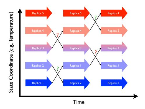
Figure 21.1.: Replica exchange schematic showing 5 replicas combined in an expanded ensemble. Large arrows represent MD trajectories of sub-ensembles while the smaller arrows represent attempted swaps between replicas in state space. Question marks represent Monte Carlo exchange attempts (green for successful, red for failed).
