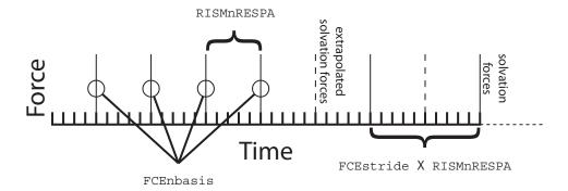
Figure 7.1.: Multiple time step methods in 3D-RISM. RISMnRESPA(=5) is the number of base time steps between application of solvation forces (exact or extrapolated). FCEnbasis(=4) is the number of previous solutions used to extrapolate forces, in this case four previous solutions. Once FCEnbasis solutions have be calculated, exact 3D-RISM forces are calculated every FCEstride(=2)×RISMnRESPA time steps; solvation forces are otherwise obtained through extrapolation.
