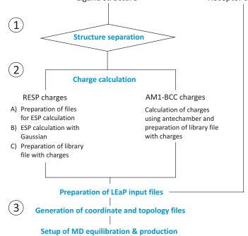
Figure 34.2.: Graphical illustration of the steps conducted for setup of MD simulations. Steps that can be executed independently by separate calls of FEW.pl are indicated by numbers. However, the individual steps can be combined, so that the whole MD simulation setup can be conducted in 1 or 2 steps for the AM1-BCC and RESP charge option, respectively (see 34.3).
